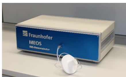
Picture 4 Photo of the developed IMS demonstrator with an attached mouthpiece for analysis of biomarkers in exhaled air.
