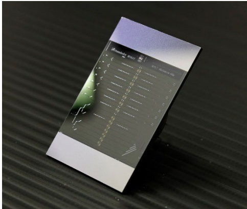
Picture 5 Integrated waveguides in silicon technology fabricated on 200-mm silicon wafers and used in combination with a functionalized surface as highly sensitive biosensors.
