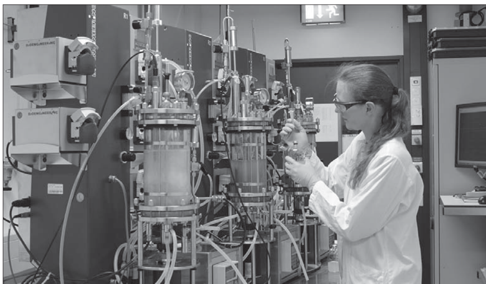
Fraunhofer is producing alcohol and acetone at its fermentation facilities, using the synthesized gas from the steel plants. Fuels and specialty chemicals can be procured from these. (© Fraunhofer IME) | Picture in color and printing quality: www.fraunhofer.de/press
