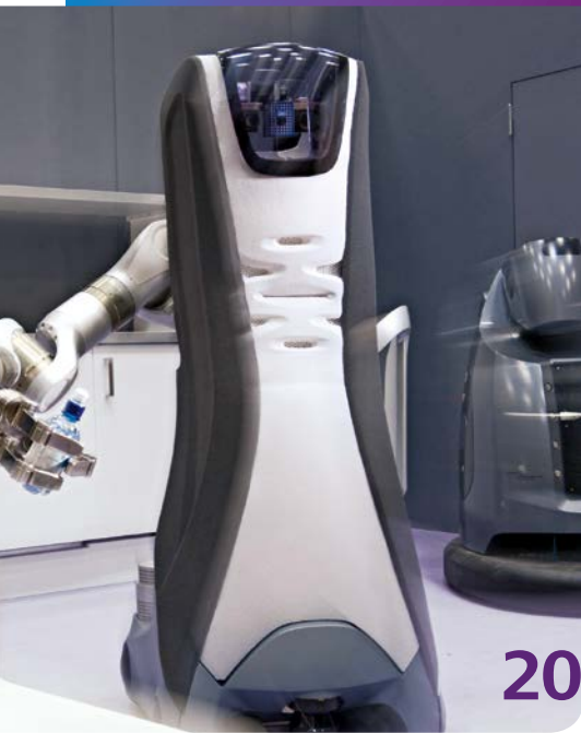
The Care-O-bot of the Fraunhofer Institute for Manufacturing Engineering and Automation IPA is the product vision of a mobile robot assistant for actively supporting people in a domestic environment.
