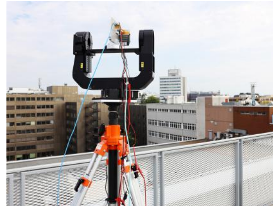
Wireless data transmission in the 155 to 175 Ghz frequency range
